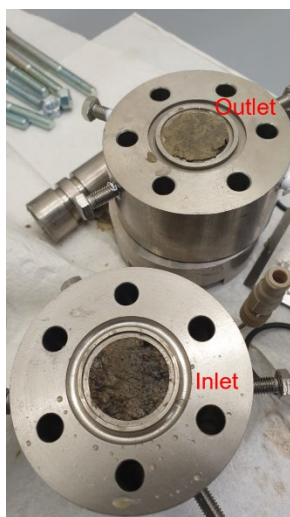
Figure 4. Columns after few days of use. Difference in the dispersion of the filling materials was observed.
