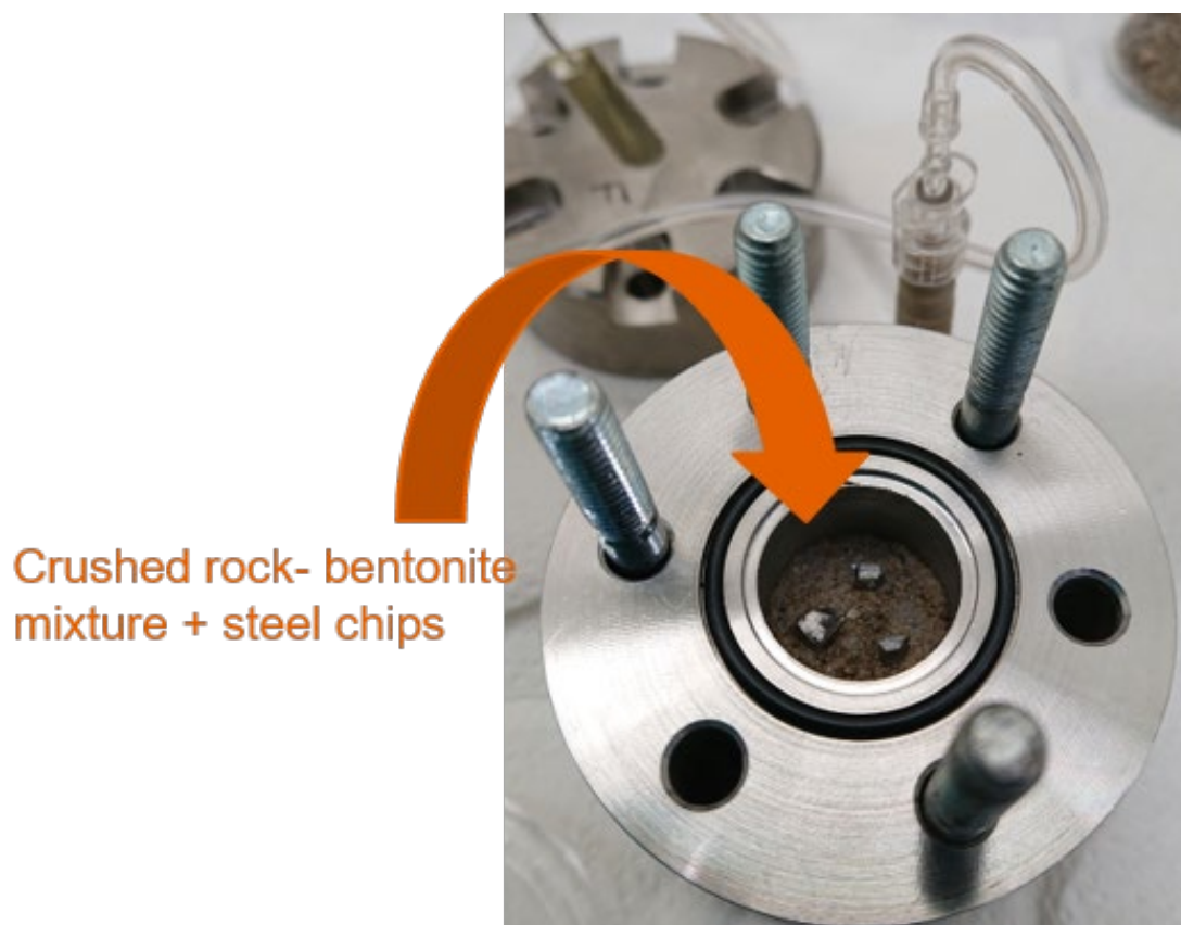
Figure 2. Example of column filling.
