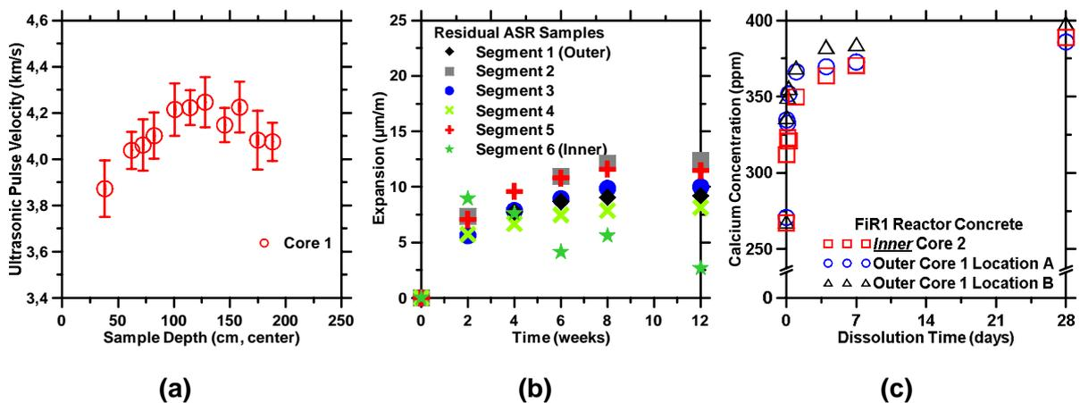
**Figure 2:** (a) Ultrasonic pulse velocity test results as a function of depth from the exterior of the concrete for core 1 (representative), (b) residual expansion data for segments of core 3 (numbered 1-6 from the surface to the interior), and (c) calcium concentration during dissolution experiments, for powders collected from the outer portions of core 1 and 3, compared with the inner portion of core 2 (e.g., lowest and highest radiation dose).
