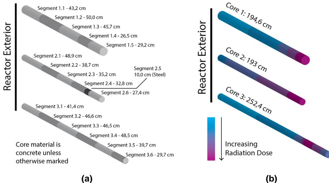
**Figure 1: (a)** Dimensions of the segments from each of the three concrete cores extracted from the FiR 1 research reactor shield, and **(b)** simulated radiation dose along each core.
